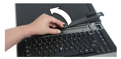
13 Lift the back edge of the keyboard slightly, then slowly slide it toward the LCD panel to release the keyboard retaining tabs located on the front of the keyboard.
